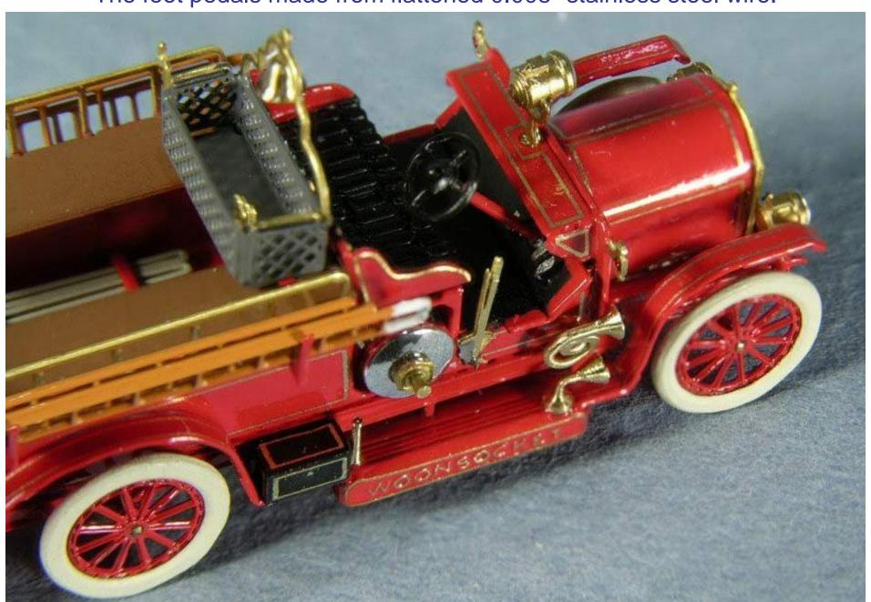
The fire extinguishers were turned from 0.060" styrene rod, and 0.010" brass wire painted black with a brass tip was used for the hose.
